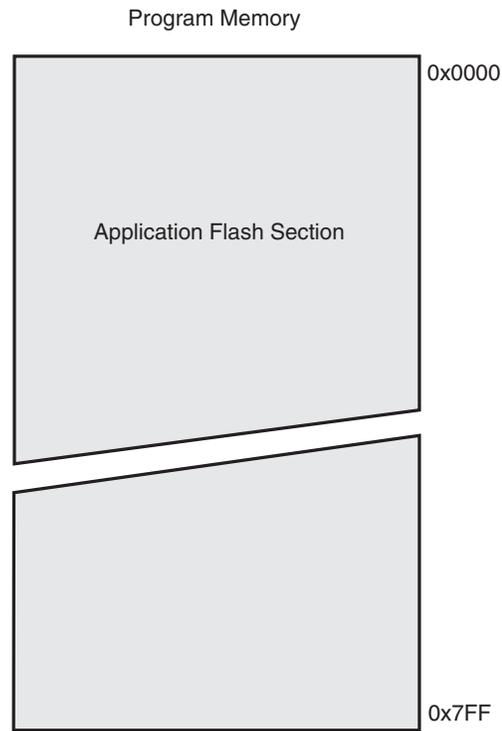
**Figure 7-2.** Program Memory Map, ATmega88 and ATmega168
