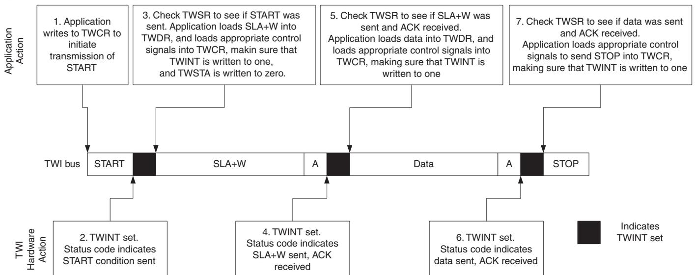
1. The first step in a TWI transmission is to transmit a START condition. This is done by writing a specific value into TWCR, instructing the TWI hardware to transmit a START
