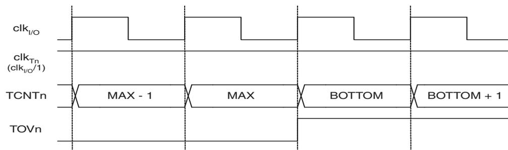
[Figure 17-9](#) shows the same timing data, but with the prescaler enabled.
