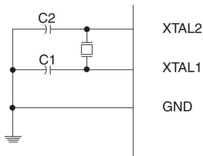
The Low Power Oscillator can operate in three different modes, each optimized for a specific frequency range. The operating mode is selected by the fuses CKSEL3..1 as shown in [Table 8-3](#) on page 29.
