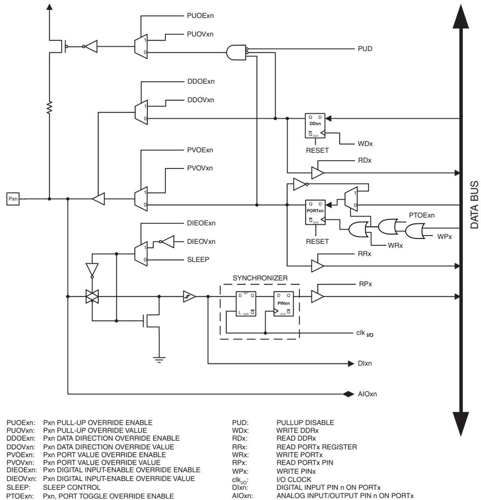
Note: 1. WR<sub>x</sub>, WP<sub>x</sub>, WD<sub>x</sub>, RR<sub>x</sub>, RP<sub>x</sub>, and RD<sub>x</sub> are common to all pins within the same port. clk<sub>I/O</sub>, SLEEP, and PUD are common to all ports. All other signals are unique for each pin.
