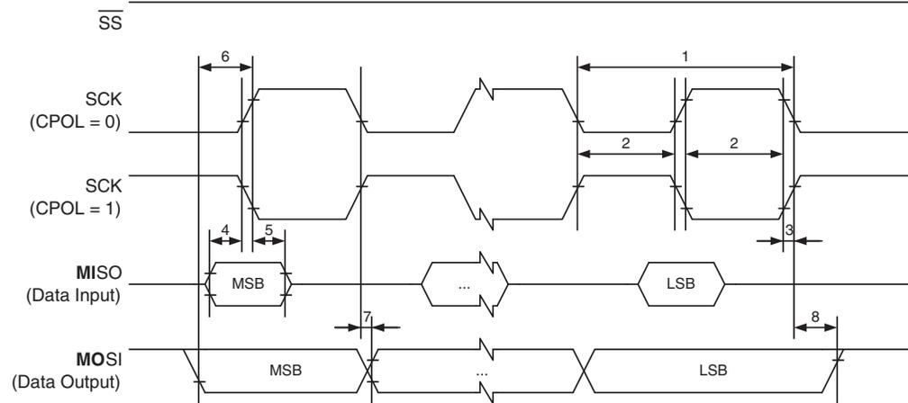
**Figure 28-6. SPI Interface Timing Requirements (Slave Mode)**
