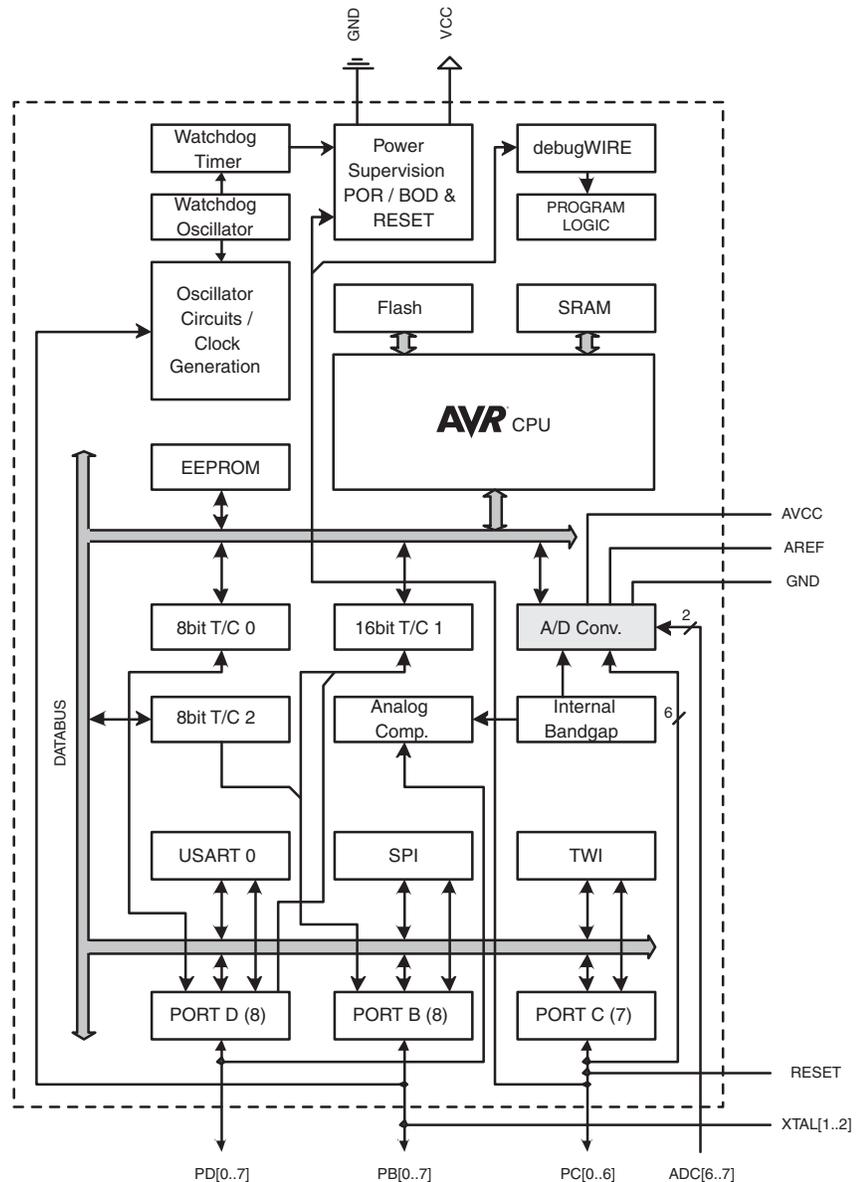
The AVR core combines a rich instruction set with 32 general purpose working registers. All the 32 registers are directly connected to the Arithmetic Logic Unit (ALU), allowing two independent registers to be accessed in one single instruction executed in one clock cycle. The resulting
